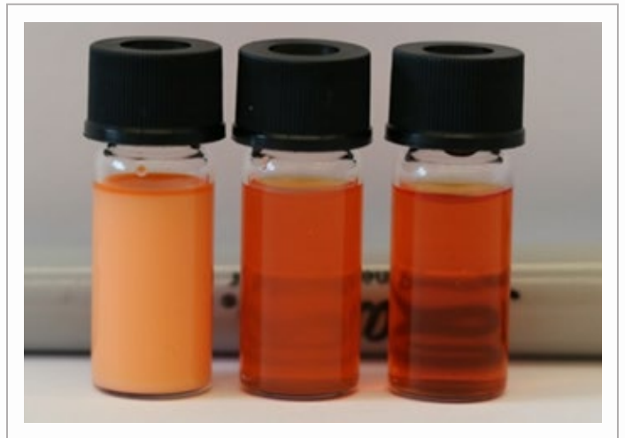
Nanoemulsions produced with varying levels of surfactant-to-oil ratios. Altering the surfactant-to-oil ratio within nanoemulsions alters particle size.
